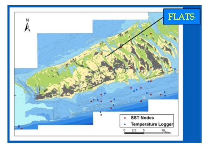
Five data loggers were installed in the passes under the bridges. The intent was to capture data from potentially very warm water generated in the flats as it passed to the south.
